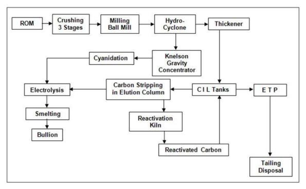
Figure 1-1: Illustrates a simplified flow sheet (Gravity-CIL cyanidation)
