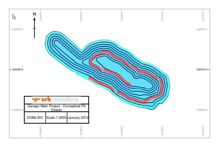
Figure 17-4: Plan View of Ganajur Main Pit Design
