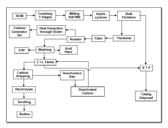
Figure 19-2: Simplified process flow sheet (flotation-roasting-CIL Cyanidation)
