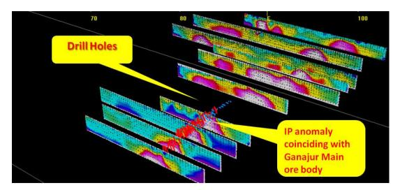
Figure 26-2: 2D Inversion model done by DESPL
