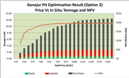
Figure 17-1: Sensitivity Curve of Pit Optimisation Result
